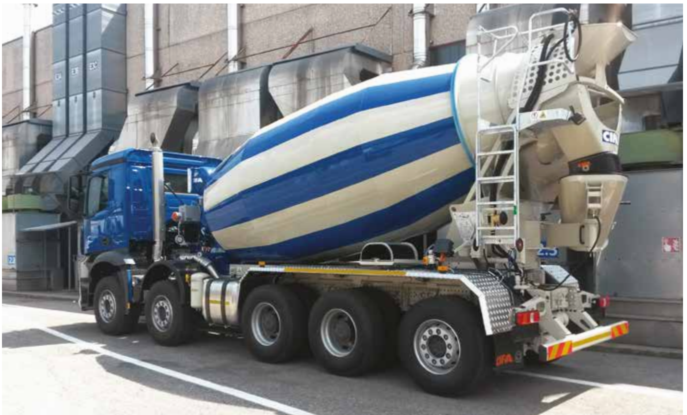
SL 12 Mudguards in aluminium for 3 rear axles (tridem), mono-support arm for discharging chute, positioning of rear control panel on the rear of left side, special support placed at 90° for chutes under the drum, loading hopper with straight rear side shape.
