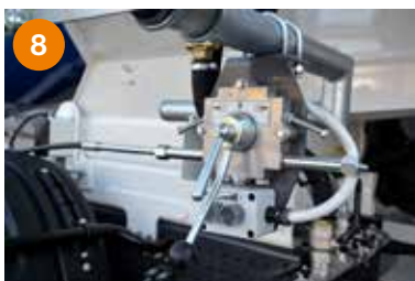
8 Manual control system driven by flexible cables (for Basic version mixer).
