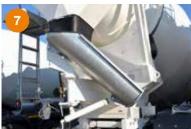
7 Hot galvanized discharge chute. One-piece type, length 1200 mm.
