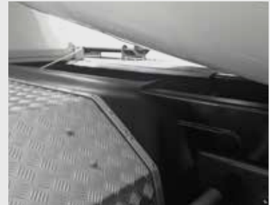
Rubber cover protection between aluminum mudguards and mixer frame.
