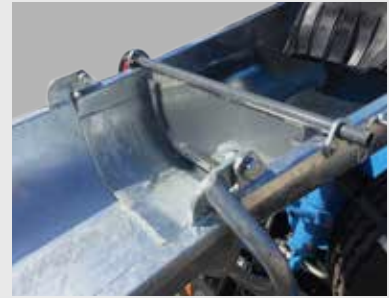
Concrete chute flap.
