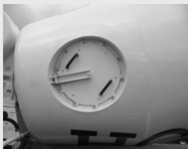
Quick release hatch for easy maintenance of the drum.
