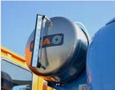
Aluminum pressurized water tank (capacity from 200 to 950 liters).
