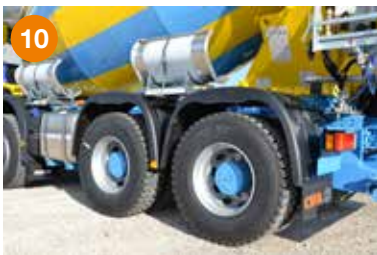
10 Polymer rear mono-axle mudguards. Double-axle mudguards made of aluminum are available on demand.
