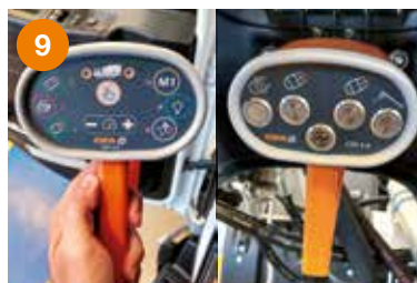
9 Electronic control system. CSD 2.0 Constant Speed Drive (for CSD 2.0 version mixer).
