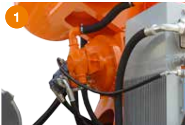
1 Water pump installed on the reducer.
