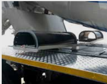
Special supports for chutes placed at 90° underneath the drum.
