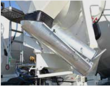
Fold over chute (1200 mm + 600 mm).
