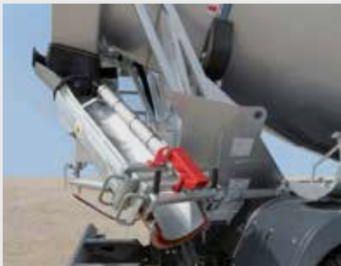
"SL 45" hydraulic extractable discharge chute.
